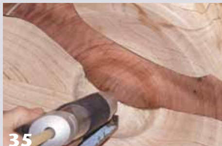
35 As wood is removed, gaps may appear between the carrier and good wood. To prevent the edges from being chipped away, use hot melt glue to fill the gaps.
