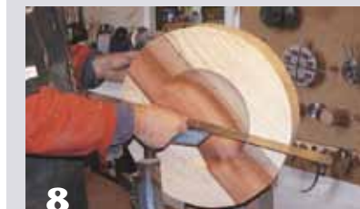
A flat base is needed for the bottom of the wings of the final piece, so check the outside surface with a straightedge.
