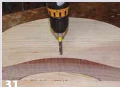
31 Drill a hole for a screw chuck for mounting the disc onto the lathe.
