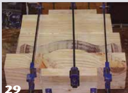
29 The carrier and good wood need to spin on a second axis, so it is necessary to build up the assembly with extra wood to create another disc.
