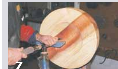
Hollow out the curved void of the underside of the piece. Sand when finished with this section.
