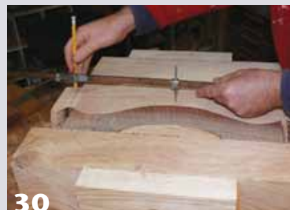
30 Mark a center for cutting out a disc. Varying the location of the center will affect the outcome of the finished piece.
