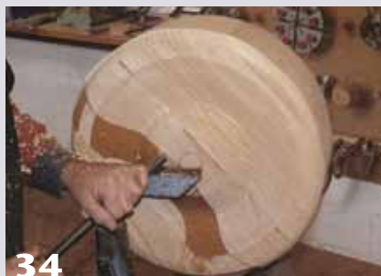
34 The disc is ready to begin shaping the front surface. The good wood will now be turned on a second axis.
