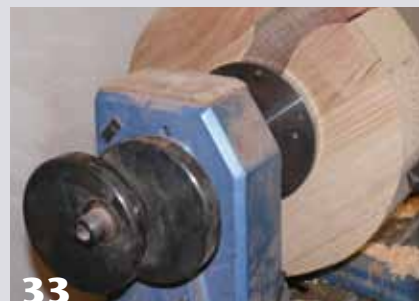
33 Because of the difference between the weight of the good wood and scrap wood, the disc may be unbalanced. My Vicmark lathe has a counterbalance that helps overcome the problem of unbalanced wood.
