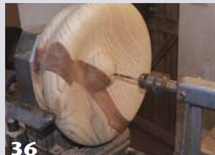
36 Finish shaping the front surface and then sand that area. Drill a hole in the center to take the screw chuck so that the piece can be reversed.
